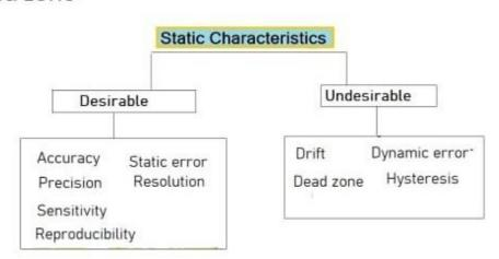
**Static Error**: The difference between the true value of the measuring quantity to the value shown by the measuring instrument under not varying process conditions.
