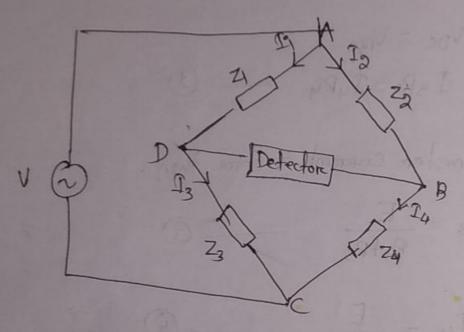
AC breidge roceinly consists of four arens, which are connected in rehombus or square shape.
