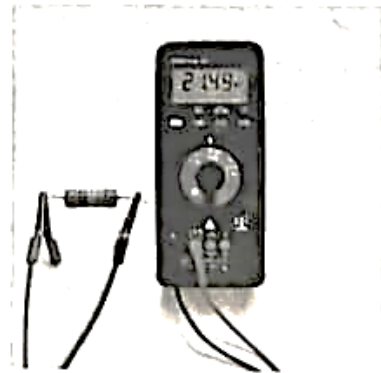
Fig. P13.2: Resistance Measurement using Digital multimeter
