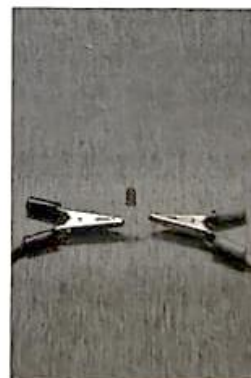
Fig. P17.2: Image showing crocodile probes connected to LED
