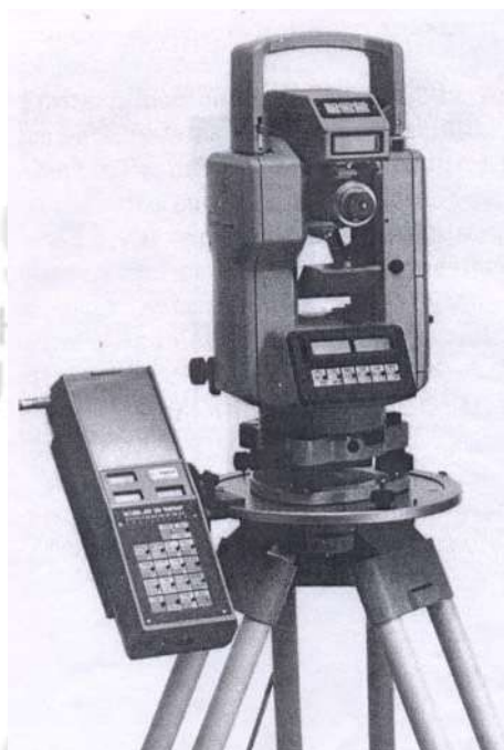
Figure 5.1 : An Electronic Theodolite with Data Collector
