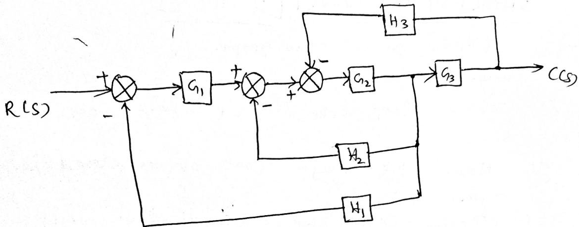
(e) Determine the transfer function of the given system.
