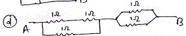
here each bit can a question of 5 marks, one has to find the Equivalent between the points A & B.
