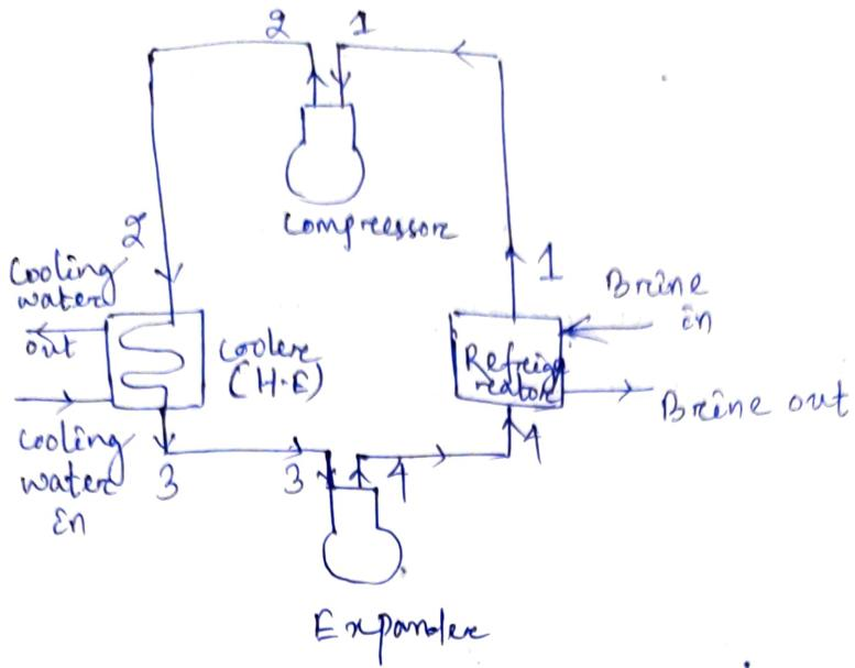
The cycle is shown on P-v and T-S diagrams. At point 1, let  $P_1$ ,  $V_1$  and  $T_1$  be the pressure, specific volume and temperature respectively: The four process of the cycle are-
