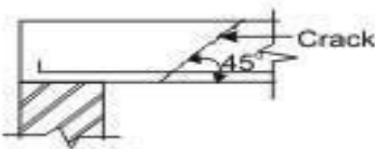
Figure 1.10 (a) Web shear progress along dotted lines
