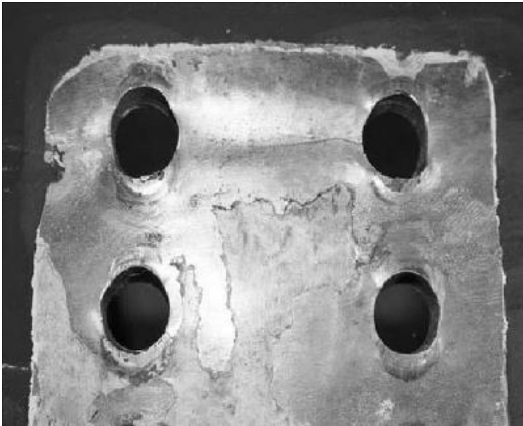
Figure 10.16 Bearing failure of plates
