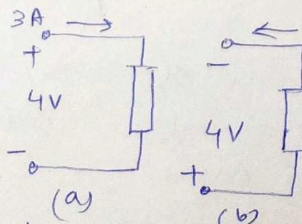
Two cases of an element with an absorbing power of  $12W$
