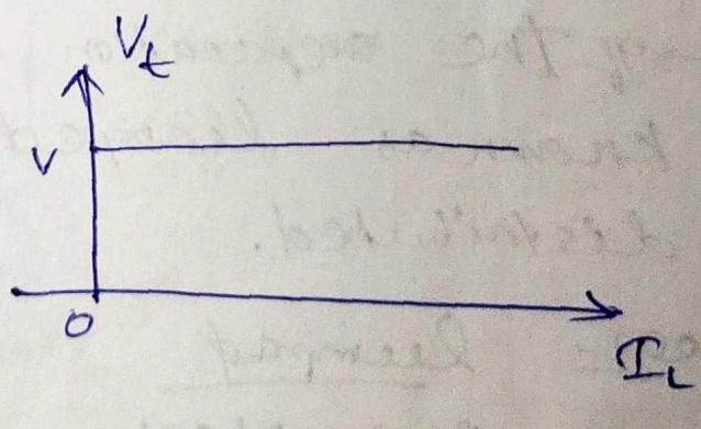
→ The terminal voltage is independent of load current or, the terminal voltage is not a function of load current is known as ideal voltage source.
