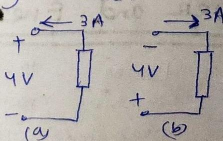
Two cases of an element with a supplying power of  $12W$ .
