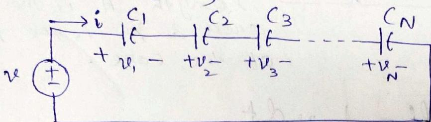
$$\frac{1}{C_{eq}} = \frac{1}{C_1} + \frac{1}{C_2} + \frac{1}{C_3} + \dots + \frac{1}{C_N}$$
