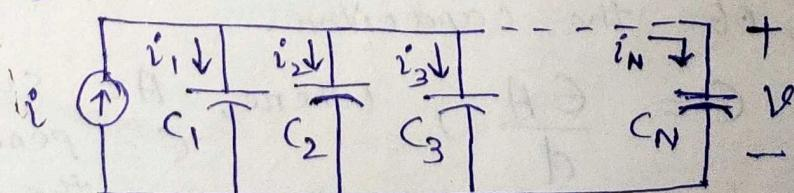
$$C_{eq} = C_1 + C_2 + C_3 + \dots + C_N$$
