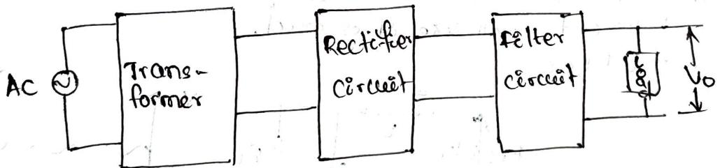
Transformer :- It converts an Ac input source to Ac required output with out changing frequency. Step down transformer reduces amplitude of Ac voltage to required level.
