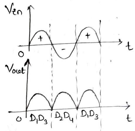
Circuit details :- The full wave bridge rectifier contains four diodes  $D_1, D_2, D_3$  and  $D_4$  connected to form bridge as shown in fig. The a.c supply to be rectified is applied to the diagonally opposite ends of the bridge through the transformer. Between other two ends A and B the load resistance  $R_L$  is connected.
