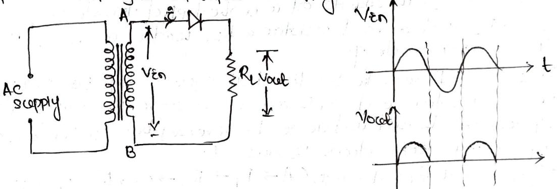
Circuit details: It consists of a diode, a transformer and load resistance  $R_L$ . Generally ac supply is given through a transformer.
