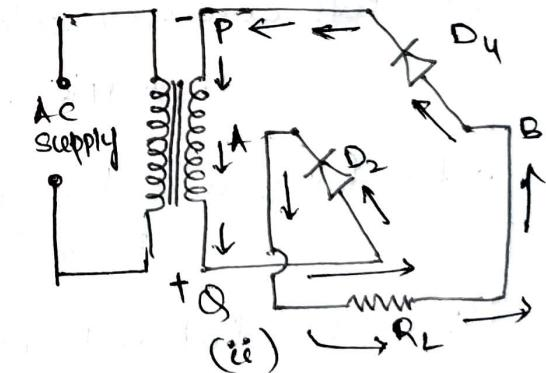
→ During negative half cycle of secondary voltage, the end P becomes negative and end Q becomes positive. This makes Diodes  $D_2$  and  $D_4$  forward biased and diodes  $D_1$  and  $D_3$  reverse biased. Therefore only diodes  $D_2$  and  $D_4$  conduct. The current flows through  $Q \rightarrow D_2 \rightarrow A \rightarrow R_L \rightarrow B \rightarrow D_4 \rightarrow P \rightarrow Q$  as shown in fig (ii).
